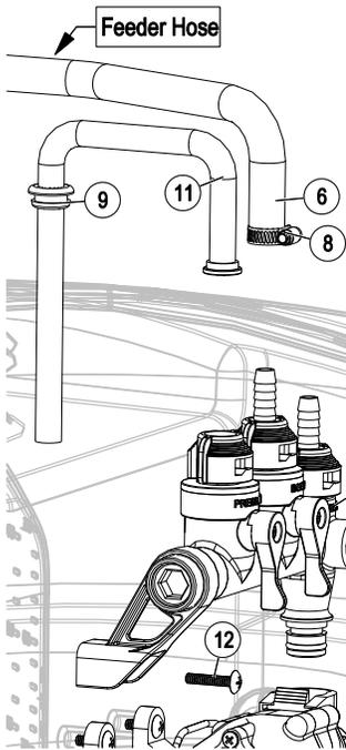
With your pump (Not Included) mounted on the 'side' of your tank this will be your plumbing configuration/setup. You may need to punch or drill the hole for your return line, approx. 13/16".
