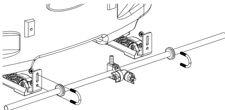
Attach the boom to the boom mounting brackets with the (2) u-bolts and (4) whiz locknuts. Make sure the u-bolts are positioned within the grooves of the grommets on the boom tube
