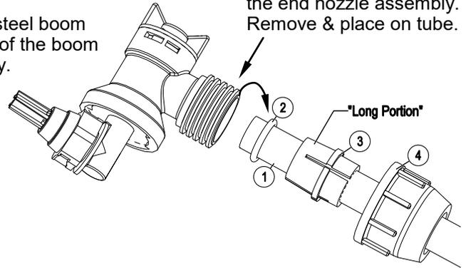
NOTE: If water is shooting back on the boom tube, item 2 is not in the correct placement.
