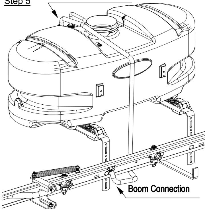
After your nozzle harness is attached to the boom, locate the 48" hose and the (2) hose clamps from the parts bag.
