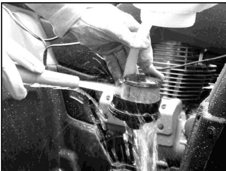
Each HGSR spray gun has a built-in filter in the spray tip. Unscrew the red spray tip holder from the lance nut to expose the tip filter. Pull the lance nut back to reveal the filter. Rinse under a hose and replace the filter element in the spray tip (the dished side faces toward the trigger).
