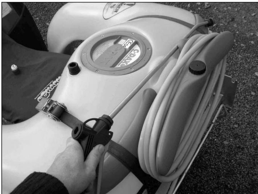
Connect the Sprayrider™ electrical connector (at front of the tank) to the battery cable.
