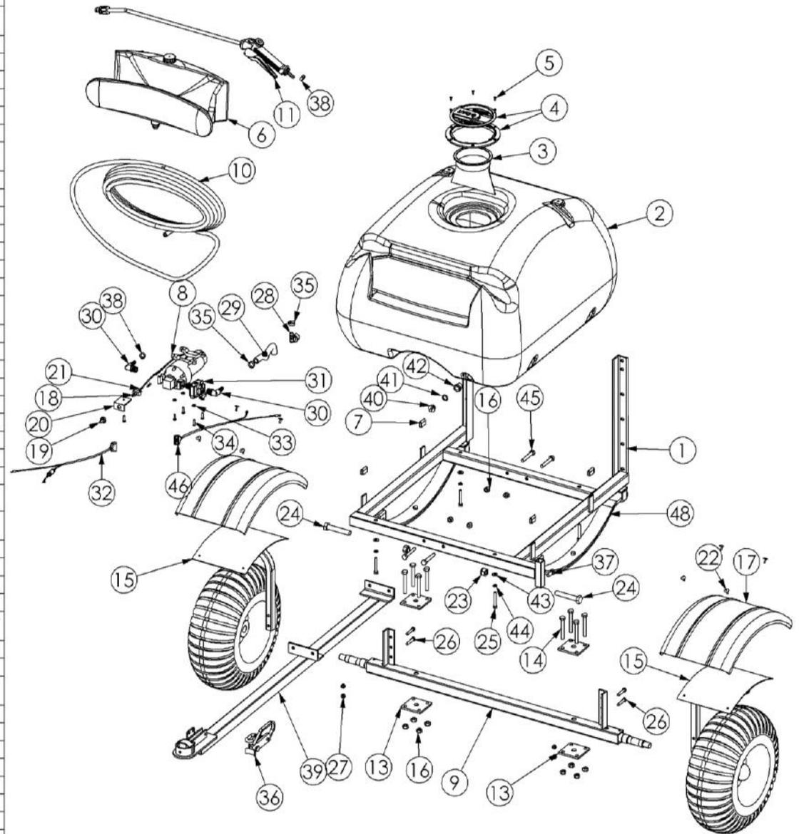
**Item 8\*:** Units manufactured prior to Jan 2015 fitted with pump 6800-5000, Pump-Flojet-Triplex-12 Volt-7.6LPM-Quad Ports.
